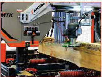
Laser sight for cutting line
